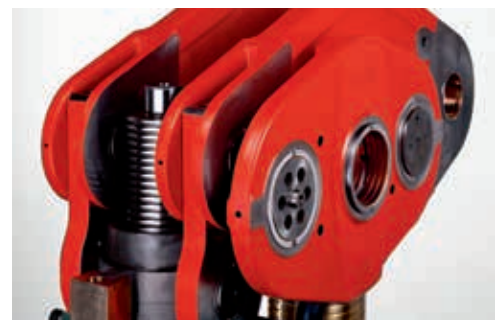
Ram adjustment during operation under production conditions.
