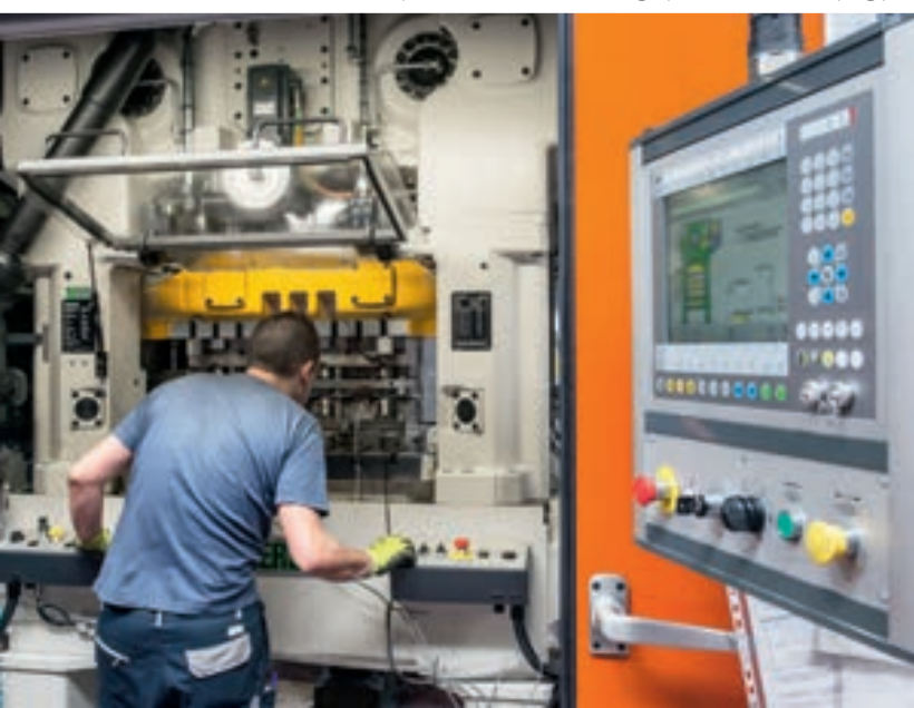
3-shift operation: BSTA 810-145 high-performance stamping press.
