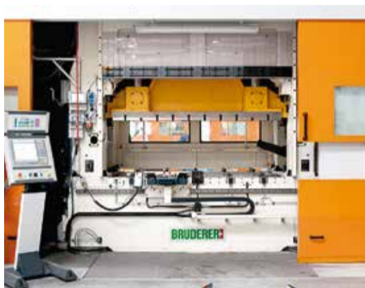
With a bed length of 2700 mm, the BSTA 2500 fully-automated stamping press has plenty of room for long tools.
