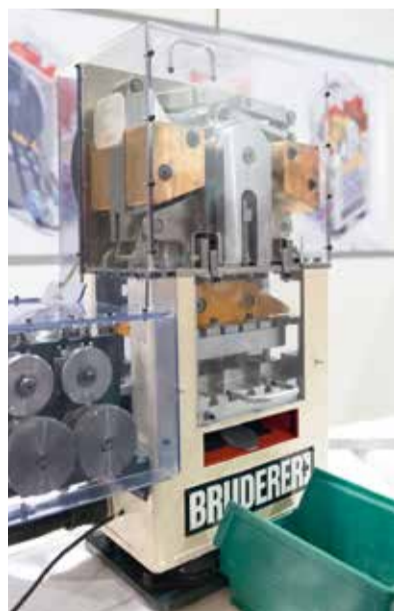
BRUDERER trainees at the OBA trade information fair presented a miniature version of a fully-automated stamping press which they had designed and built themselves.
